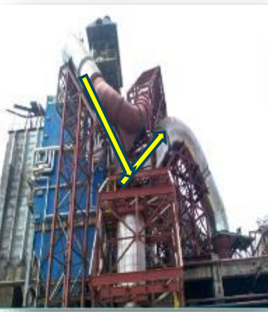
AQC : Booster Fan Bypassed Route After Modification
